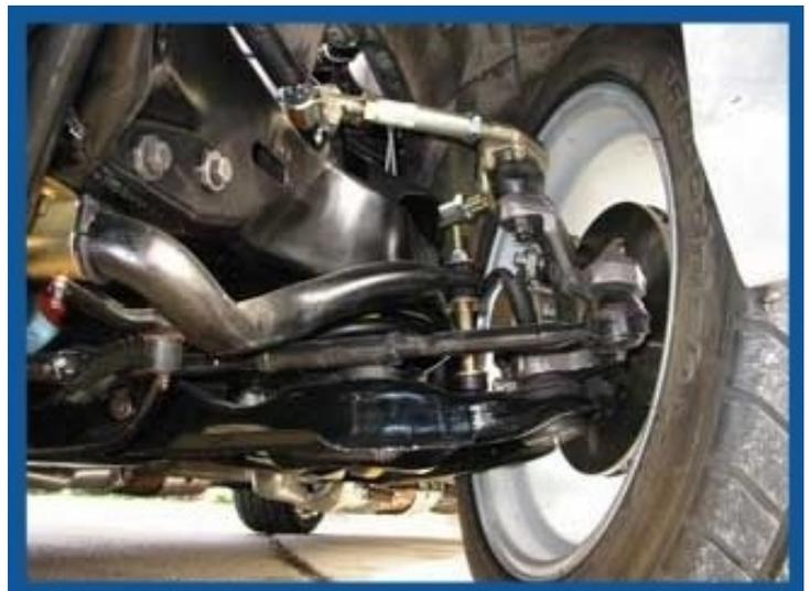
Chevelle suspension using stock spindles, Howe Precision tall ball-joints, and SPC adjustable upper arms from SC&C.
