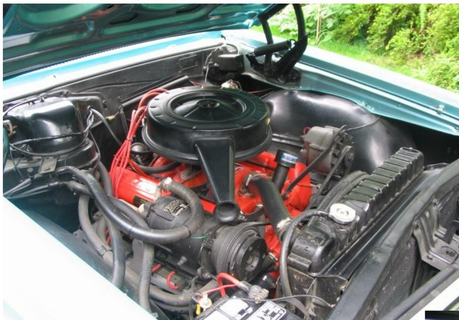
He ordered this car with factory air, a SS interior and the power pack 220hp 283 V8. He switched the manifold over to a two barrel carburetor setup when the gas prices changed in the mid 1970's. I have the original manifold but the 4 barrel carburetor is shot. After some hard fought convincing I talked him into selling me the car and I drove it back to Minnesota with 70,000 original miles.
