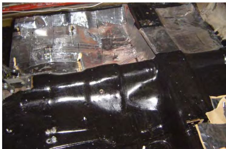
Hushmat insulation installed over POR-15 on passenger side
