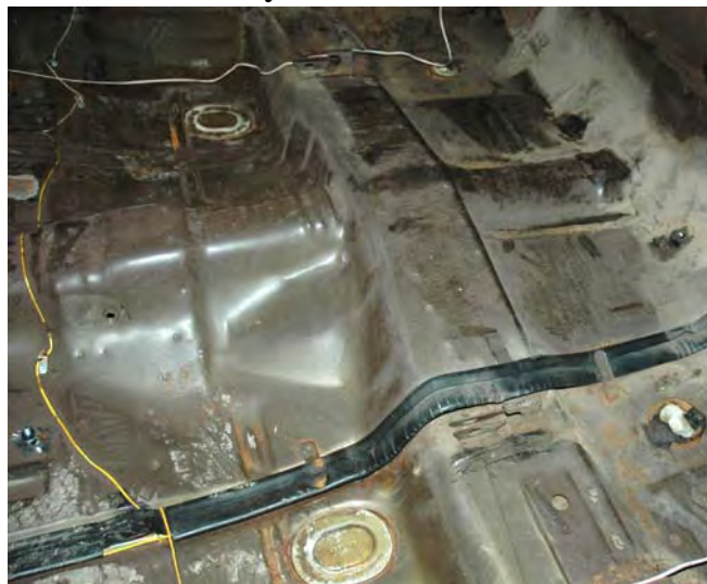
Original sound deadener removed and vacuumed
