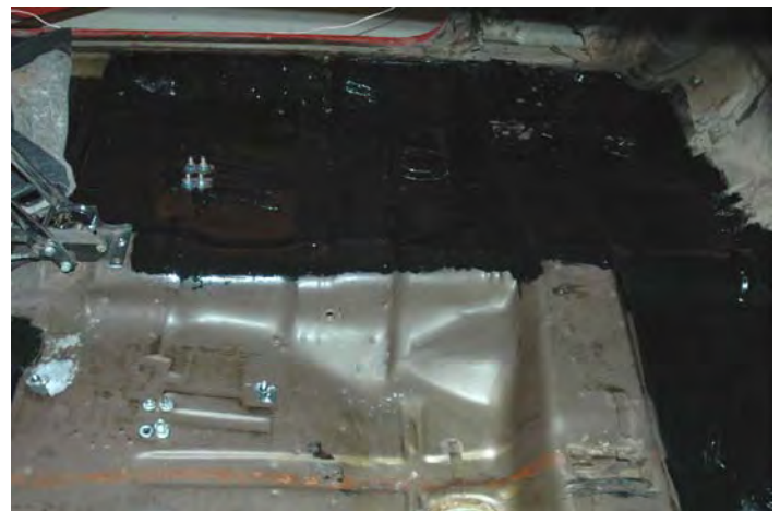
Prepped floor with coating on passenger side
