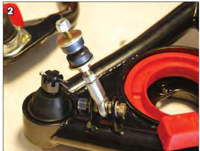
2. Additionally, the control arms employ urethane bump stops on both uppers and lowers, and the sway bar link is adjustable with a spherical rod end at the control arm mount. Grade 8 hardware is used throughout.
