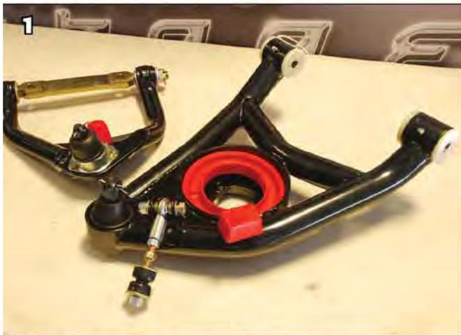
1. Each set of front control arms from TRSD features heavy-wall tubular construction to help shed a few pounds of unwanted weight from the front of your Chevelle, while providing additional structural rigidity. The ball joints are already installed in the precision pockets found on each arm.
