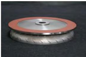
The pinkish friction surface you see here is the torque converter's lock up clutch on the back of the turbine. If your converter is a lock up unit (many actually aren't), at a certain RPM in top gear the torque converter will lock up thanks to this friction surface, and the torque converter can no longer slip. This is a good thing because now all of the engine's power will get transmitted through the transmission and none will be wasted, helping with gas mileage and drivability.
