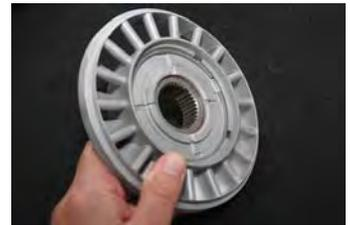
The stator is the brains of this operation. TCI tells us, "The stator changes fluid flow between the turbine and the pump, which is what makes a torque converter a 'torque multiplier', and not just a fluid coupling."
