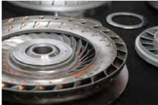
The turbine side of the converter that is bolted to the flex plate will always spin at the same speed as the engine, while the pump side will slip to a certain point and let the engine keep turning, while you come to a stop. Once the engine reaches a certain RPM, the fluid will be moving fast enough through the torque converter that the two sides will begin to couple and the car will start to move forward. The point that the car begins to move is known as the “stall speed.”
