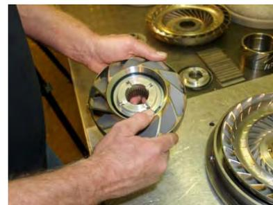
Stators are selected with specific characteristics – the number of windows and the angle of the fins are important depending on your application.
