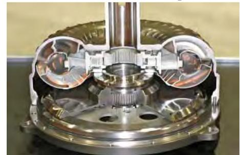
**Left: TCI's 9.5 and 10-inch Pro-X converters are used in classes like X275, where Jason Lee and Bob Kurgan have used them with great success. Right: One of TCI's lockup converters designed for use with the 6L80E transmission found behind many LS engines. It uses a fluid-activated clutch to assist in lockup.**
