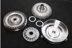
Torque converters come from the factory welded up, so it's pretty hard to get a look inside and see what makes them tick. From the right counter-clockwise, you can see the cover (which bolts to the flexplate), the impeller pump (which slides over the transmission input shaft) the turbine, and the stator.
