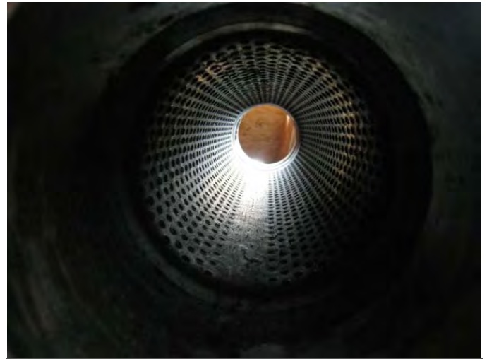
While straight-through exhaust mufflers look like the gases and noises go straight through the muffler, there is actually a lot going on inside there.
