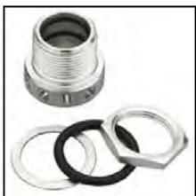
Ever looked at buying new valve covers and thought, those pare exactly what I want, except I need a breather? Summit Racing has a solution. Their kit includes the baffle, a locknut, o-ring, and sealing washer. Simply drill a 1.375" hole in the position you need, slip it in and tighten the locknut. It accepts most breathers that fit a 1.00" ID hole. At \$25.95, it's not exactly dirt cheap, but it allows you to position a breather exactly where you want it or even add an additional one.
