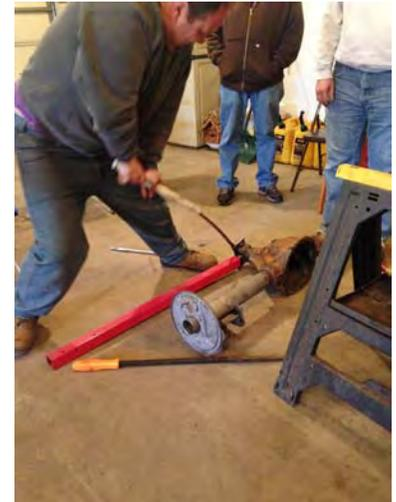
Starting the crush sleeve, note the force needed.
