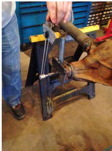
Beam type torque wrench
