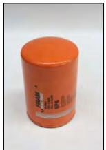
Fram's racing filters are designed to increase oil flow through the filter but this comes at the cost of reduced efficiency in terms of dirt below 30 microns. This assumes that the oil will be changed much more often on a race style engine. For this reason, race filters are not recommended for daily street use.
