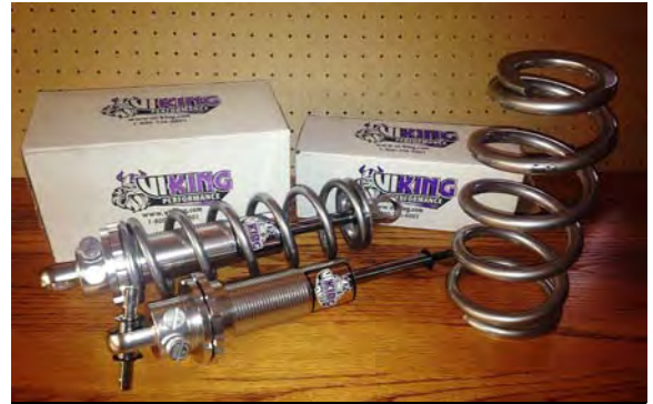
Front and Rear coilover shocks and springs. Rear has spring installed. Rear installation in an upcoming month.
