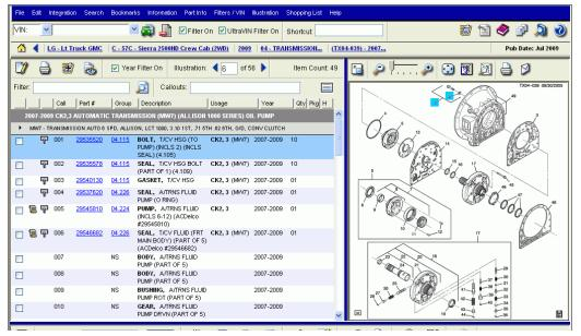
This what is the modern parts catalogs look like now. You can see the picture is for a 2009 3/4 ton HD with an Allison transmission. and a portion of the parts list associated to it. Each callout has a parts line, though not every part serviceable as indicated the NS by (nonserviceable) note. You
