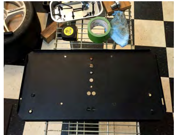
I knew I could re-use the base, just make a template and drill holes to match the TV's spacing. The larger holes in the center will become the vertical arm mounting holes.
