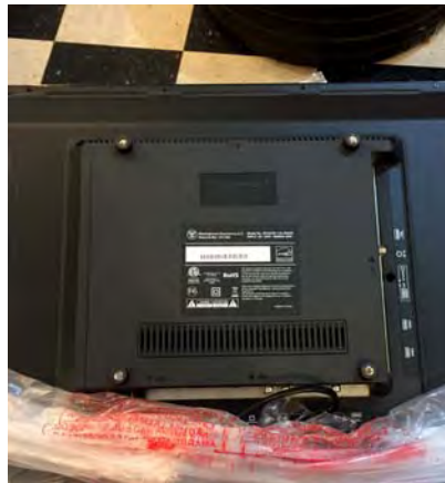
Every new TV has a wall mount style design on the back that uses threaded inserts. All you need is a way to use them.
