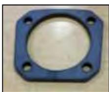
figuring, and axle sliding in and out, I realized the spacing won't ever line up right. A call to Chris P revealed that there's a guy on eBay selling spacers that will correct my problem. Not as cheap as one would hope, but once I got them and tried again, well worth the money. Yes, I could have made them, but why bother? These were done nicely.
