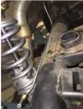
Time for hard lines. I didn't have a bending tool, so that was on the shopping list. Next were sticks of straight tubing. I picked up 4 sticks, figuring that I needed one for each side going from the tee fitting on top of the rear end pumpkin and the first ones would be practice and most likely become garbage. I also cheated and borrowed a flaring tool from work.
