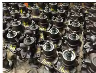
Cores come in by shipping container, get cleaned and ID'd, then disassembled. Once done, they're boxed and ready to ship.
