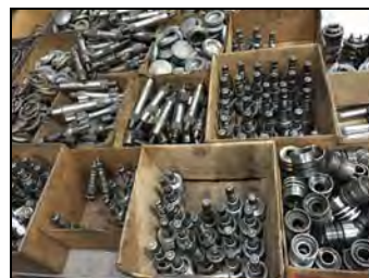
Cores come in by shipping container, get cleaned and ID'd, then disassembled. Once done, they're boxed and ready to ship.
