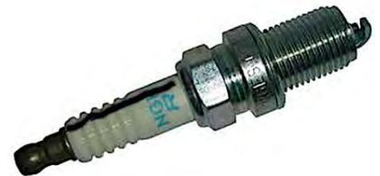
Notice how the gap side of the plug is directed to the intake valve? This provides the desired fuel mixture combustion that yields a greater horsepower output.
