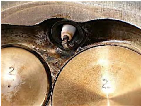
The grounding strap of this plug is shielding the electrode, and will result in a less effective burn.
