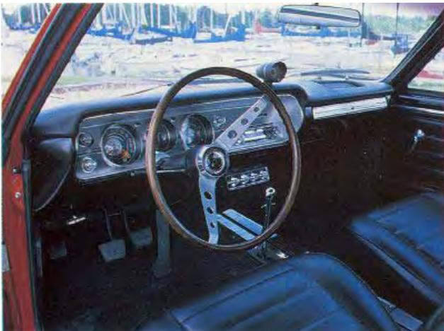
©2007 Publications International, Ltd. **Bucket seats and console were standard in the SS 396; the simulated wood steering wheel was an option, and the dash-top tach a mandatory extra.**
