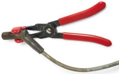
Grab hold of plug wires with pliers and you'll for sure damage the boot. But the padded jaws on this spark plug boot pliers let you get a firm grip on the spark plug boot without tearing it. Slide it onto the top portion of the boot near the wire and clamp down. That'll apply force to the metal clip inside the boot. Then twist and pull. No more torn boots or wires. You can buy the Lisle No. 52990 Spark Plug Pliers online.
