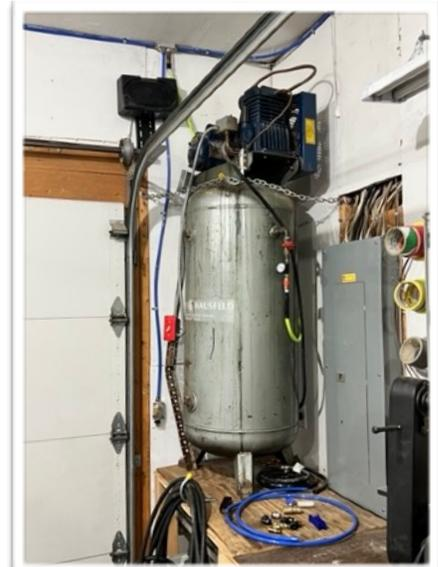
Notice the manifold at the top, the pressure gauge and main valve from the tank, and the drop down the wall. Disregard the ugly compressor. The tank is 5th owner, the top is from another that rusted out, but it works.
