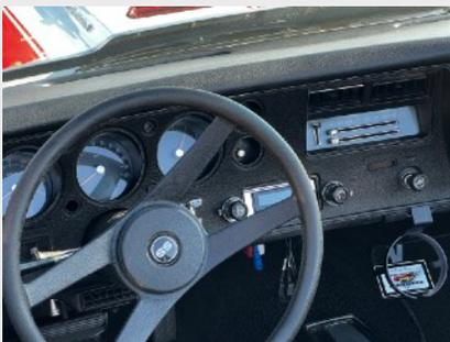
This looks to be an original '72 round gauge dash sporting the "fasten seat belts" light over there by the lighter knob. Most dashes get replaced and don't have the hole for the light. Sweep dashes have it under the speedo area.
