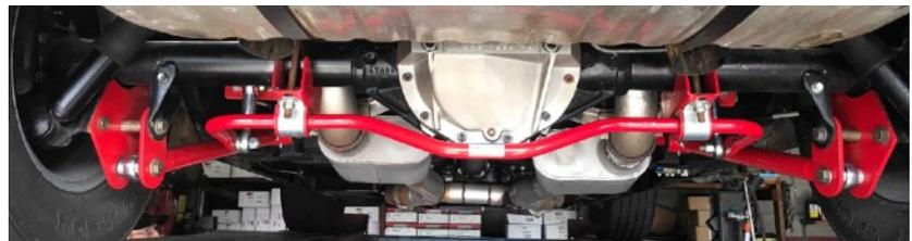
Still not my car (I chose a black kit), but you can see the mounting really well. This one isn't even a UMI product, but the idea is the same. By mounting the end links to the body/chassis, it helps lock the rear axle in place versus on turns rocking up and down.
