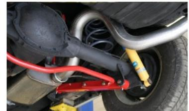
Not my car, but this is how my last sway bar mounted-just to the lower bar. If you use stock bars, make sure there's a reinforcement plate in place!
