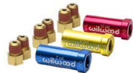
Isolation valves have a pressure light switch and measure front and rear brake pressure. If pressure drops too far it will trigger the light, but also will stop fluid flow to the area losing pressure and maintain pressure to the other side.
