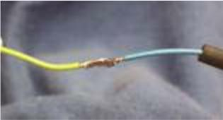
Apply solder - The solder should just FLOW right into the joint - if it doesn't it's either not hot enough, or is dirty.
