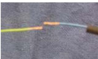
Strip off about 3/8" insulation on both wires
