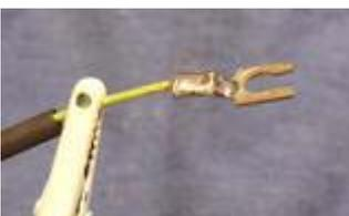
Apply heat, then solder. Again the solder should just FLOW right into the connector body.
