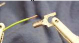
Strip the wire - NOTICE, only enough copper is exposed that will fit into the terminal
