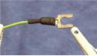
Slide the shrink tube over the connection, and heat.
