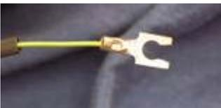
Crimp the connector onto the wire
