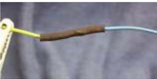
Slide shrink tube over joint, and heat - Done
