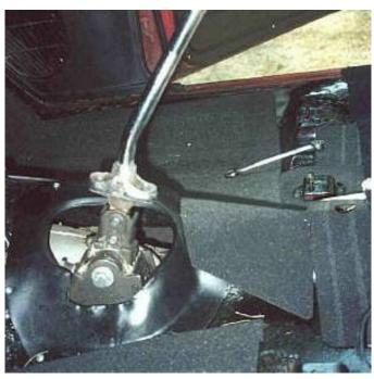
The stock Hurst handle bent back at around 11" of height and the top of the ball was about 15" off the floor; a 1 1/2 " differential. The original floor had to be trimmed to clear the left side of the Hurst box as shown.
