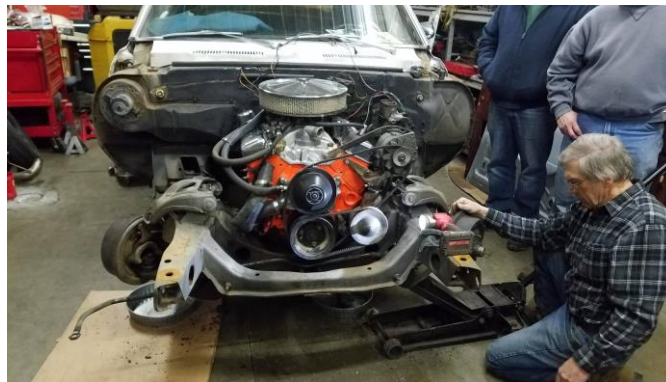
Mitch giving a few good whacks to separate the suspension.
