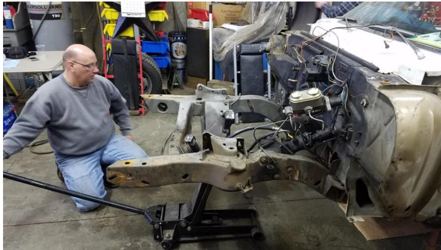
Chris setting the jack to support the sub-frame.
