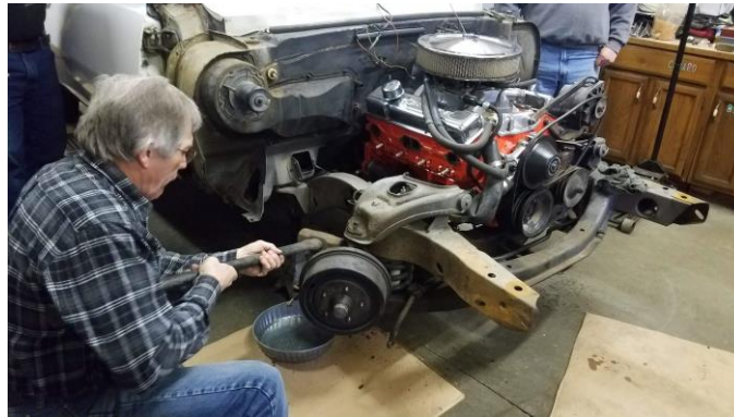
Mitch giving a few good whacks to separate the suspension.
