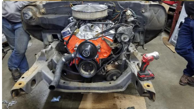
Suspension and brakes removed and onto the engine/tranny pull.
